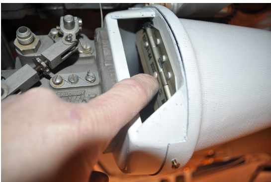
Bendix type installation, note spring actuated door without cable (builder modification).
