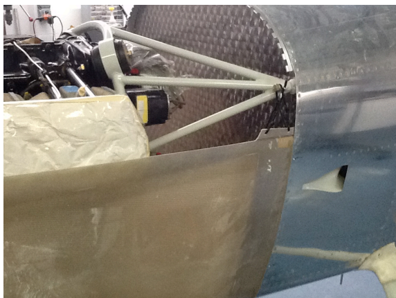
Note remaining flange strip tied into mount
